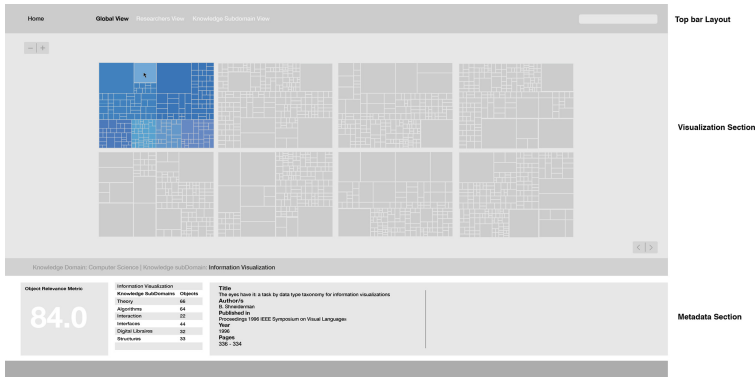
Fig. 1. Global View: a color gradient identifies the SKOs knowledge subdomain (e.g. gradient of blues). By placing the mouse pointer over the SKOs areas, a descriptive tooltip about object metadata emerges in the metadata section. The bottom left rectangle provides the object relevance value (84.0 in this example). The directional buttons inside the visualization section provide the navigation menu, and plus and minus buttons provide the zoom interactivity. (Color figure online)
