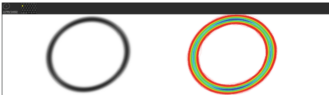
Fig. 10. General view of pillar circularity. In the right-side visualization, color gradients from red to blue represent the most common vertices in each nanopillar in crescent order. Red means less common and blue means most common vertices. (Color figure online)
