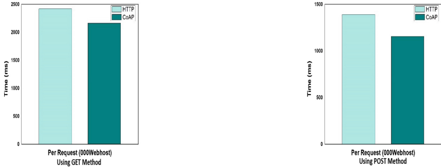
Fig. 5. Comparison of HTTP and CoAP protocols based on GET and POST method using 000webhost as a Storage.
