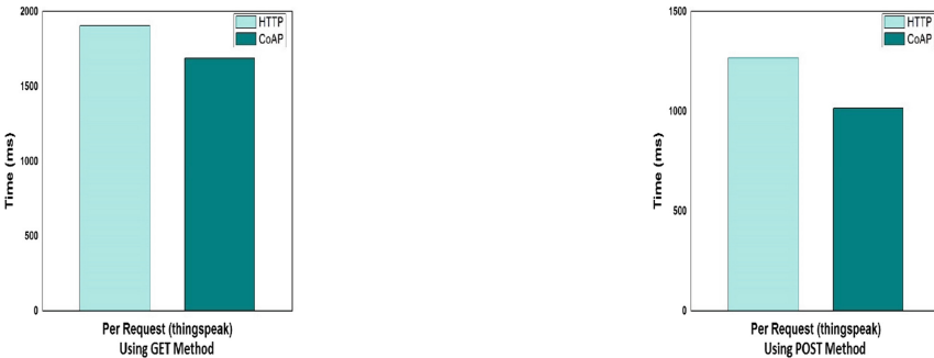
Fig. 4. Comparison of HTTP and CoAP protocols based on GET and POST method using Thingspeak as a Storage.
