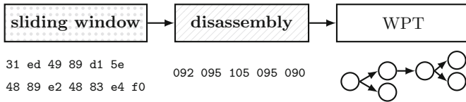
Fig. 9. The general processing pipeline during WPT-based classification.
