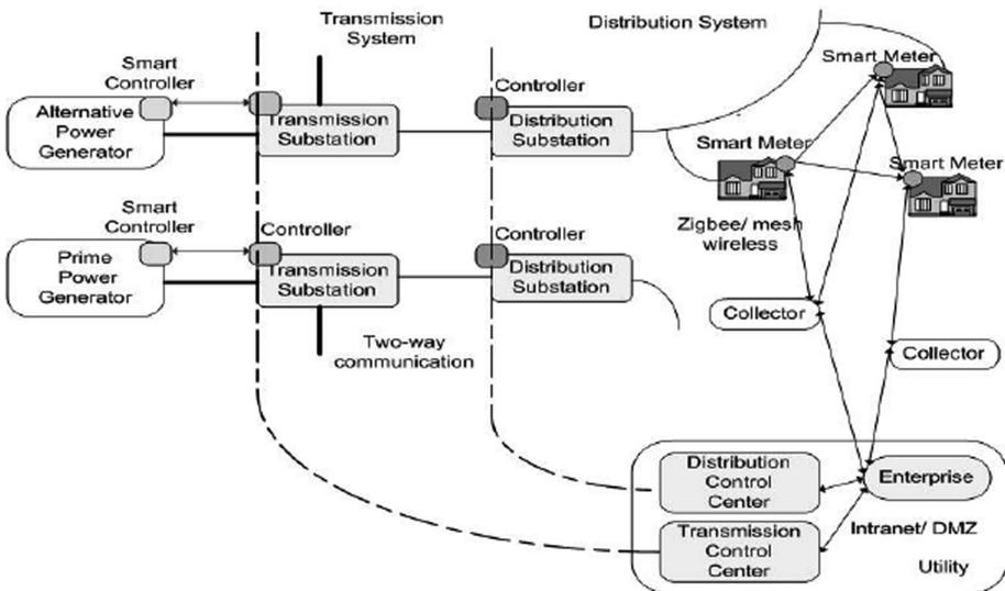
Fig. 2. Typical smart grid architecture (image source: Mavridou et al. [1])
