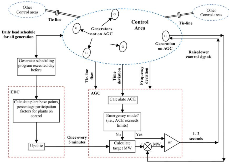
**Fig. 1.** Typical block diagram for the Automatic Generation Control. The AGC receives input signals including the *frequency deviation*. The input signals are used to calculate the *area control error ACE*, and thus determine the control signals needed to return the utility back to the normal state (image source: Hasan et al.: [4]).
