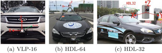
Fig. 3. Lidar placement
