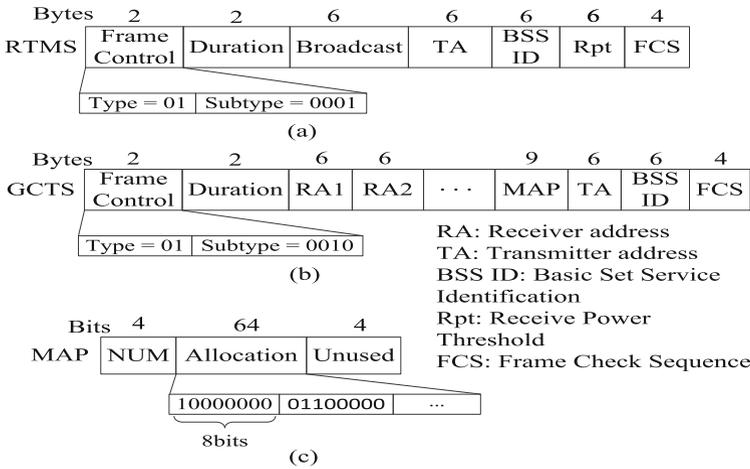
Fig. 2. Control frame structure of SCG-OFDMA.
