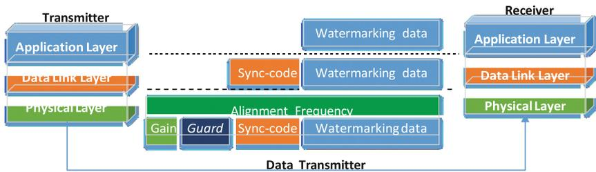
Fig. 3. The protocol stack of sound-wave transmission system
