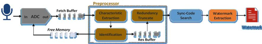
Fig. 6. The receiver of data link layer
