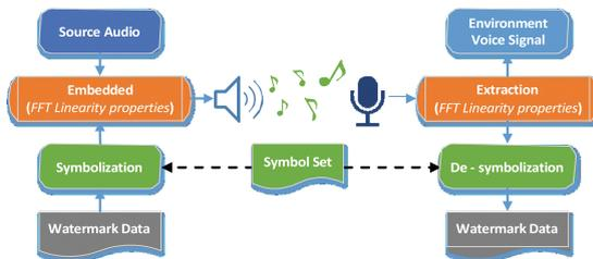
Fig. 2. Sound-wave transmission system architecture
