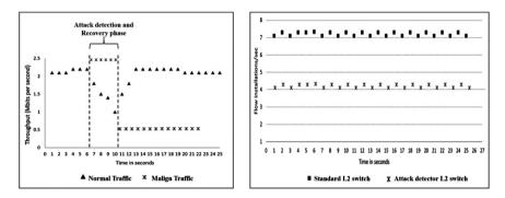
Fig. 9. (a) Link Saturation (b) controller performance
