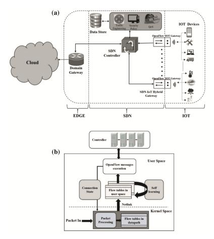
Fig. 5. (a) Tightly coupled SDN-IoT integration, (b) flow analysis in SDN-IoT hybrid device
