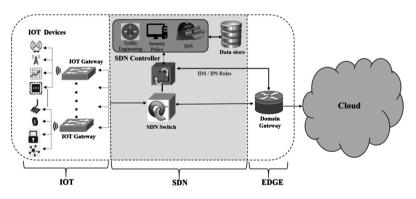
Fig. 4. Loosely coupled SDN-IoT integration
