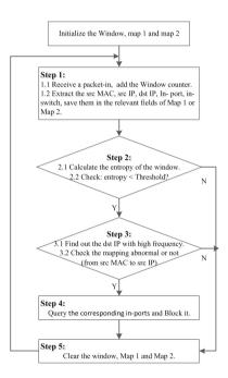
Fig. 1. The main flow chart of EDDM
