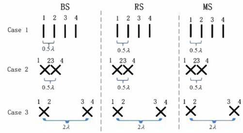
Fig. 3. Antenna configurations
