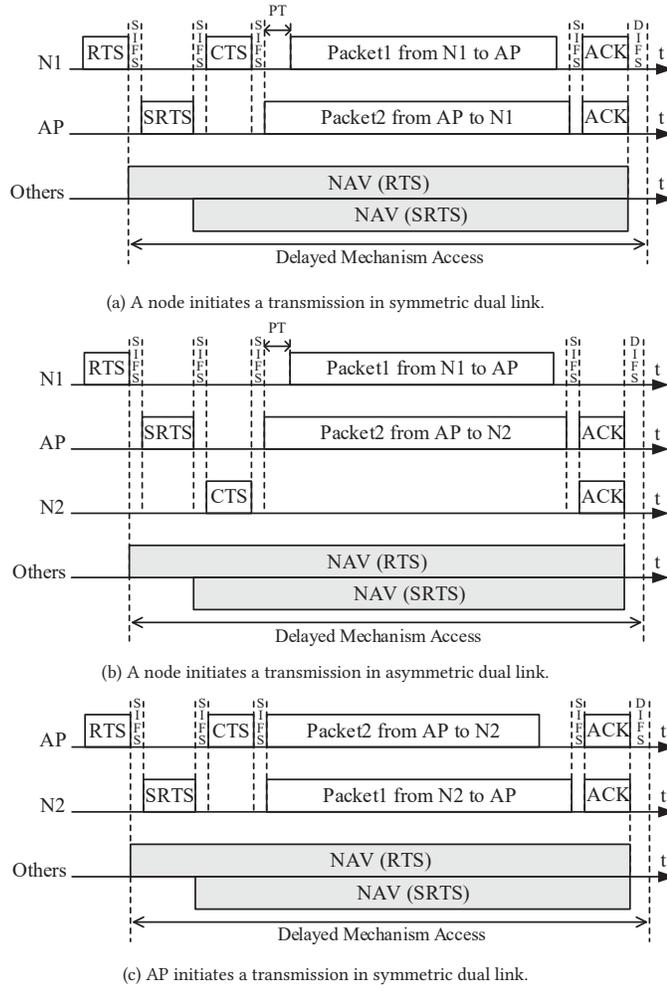
**Figure 3: Successful IBFD wireless transmissions with FDMA-CE mechanism.**
