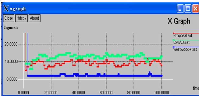
Figure 8. Slow start threshold comparison for 10% packet corruption rate
