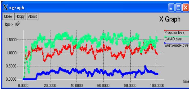
Figure 6. Bandwidth utilization comparison for 10% packet corruption rate
