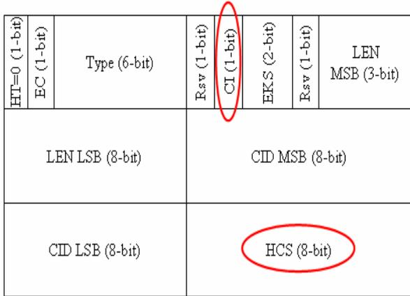
Figure 2. Format of IEEE 802.16 MPDU header
