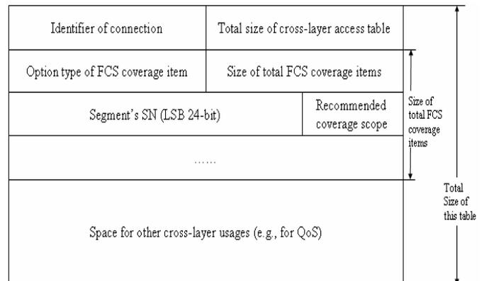
Figure 3. Format of “cross-layer access table”
