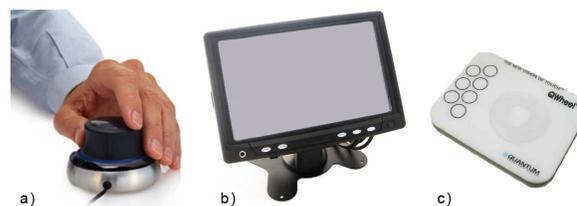
Figure 1: The three input devices we used in our user tests: multifunction knob, touchscreen and wheel slider
