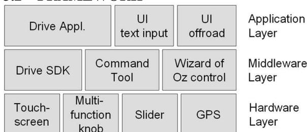
Figure 2: The framework of the testing system
