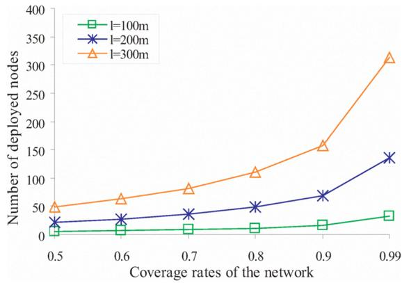
Fig. 3. Comparison of coverage under different network sizes.
