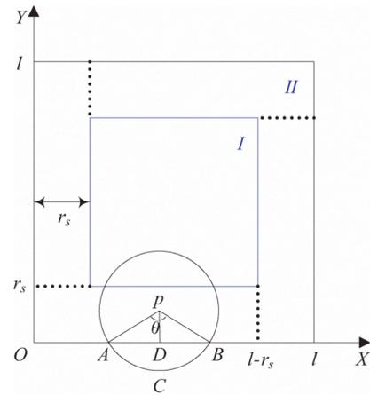
Fig. 1. Illustration of a sensor node  $p$  that is located in Region II.  $O$  is the origin of a coordinate system.  $A$  and  $B$  are the intersection points between the sensing disk of node  $p$  and the border of the network region.
