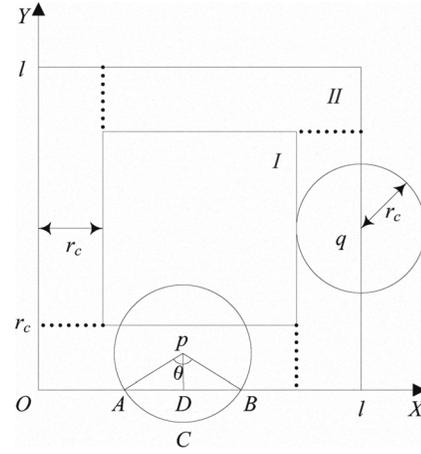
Fig. 2. Illustration of a sensor node  $q$  that is located on the outer border of Region II.  $O$  is the origin of a coordinate system.  $A$  and  $B$  are the intersection points between the sensing disk of node  $p$  and the border of the network region. Node  $q$  is located in the border of the network region.
