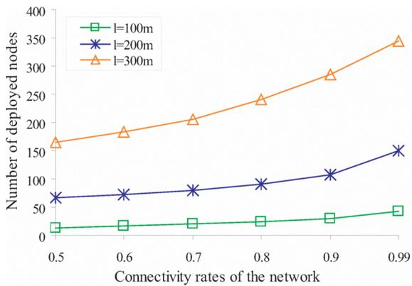
Fig. 4. Comparison of connectivity under different network sizes.
