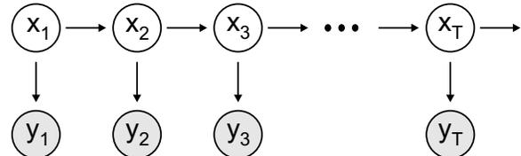
**Figure 2: State space model for the proposed location sensing system. Clear circles indicate hidden state variables, grayed circles indicate observations, horizontal arrows indicate state transition functions and vertical arrows indicate observation functions.**
