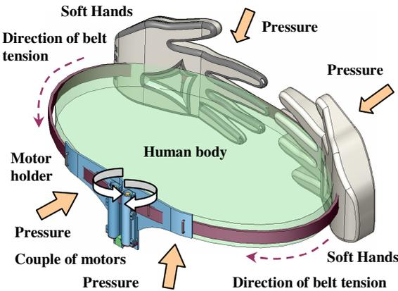
Fig. 2. Structure of wearable HaptiHug device
