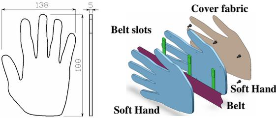
**Fig. 3.** Left: Soft Hand dimensions. Right: sandwiched structure of Soft Hands.
